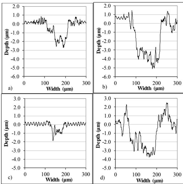
Fig. 3. Profilograms traces worn on irradiated titanium samples a) at a fluence of  $1 \times 10^{14}$  Xe/cm<sup>2</sup> – stage 1, b) – stage 2, c) at a fluence of  $5 \times 10^{14}$  Xe/cm<sup>2</sup> – stage 1, d) – stage 2.
