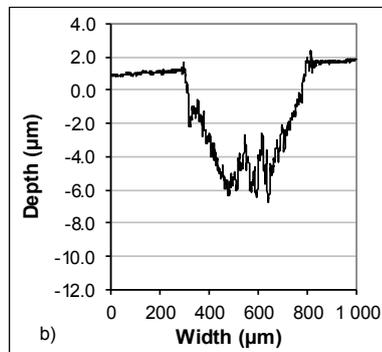
Fig. 4. Profilograms traces worn on irradiated titanium samples a) at a fluence of  $2.2 \times 10^{14}$  Xe/cm<sup>2</sup>, b) at a fluence of  $5 \times 10^{14}$  Xe/cm<sup>2</sup>
