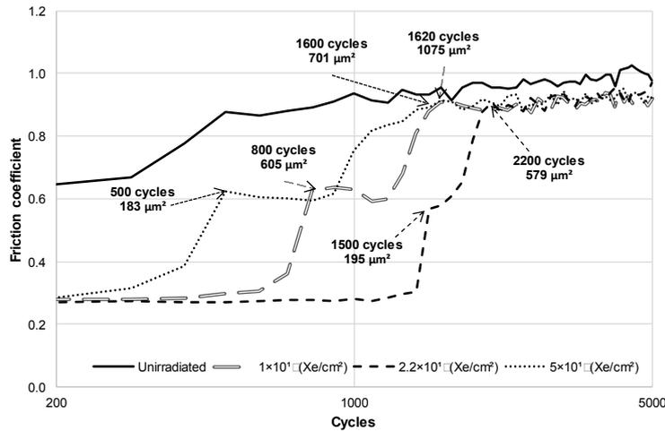
Fig. 2. Change in the titanium friction coefficient and tribological wear depending on the number of tribological test cycles
