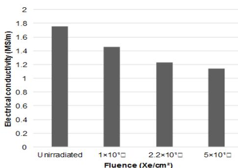
Fig. 6. Results measurements of electrical conductivity of titanium samples
