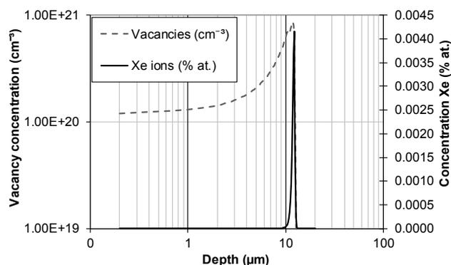
Fig. 1. SRIM calculations of Xe ion distribution profiles (168 MeV) and radiation defects in the titanium sample. The fluence in both cases was  $2.2 \times 10^{14}$  Xe/cm<sup>2</sup>
