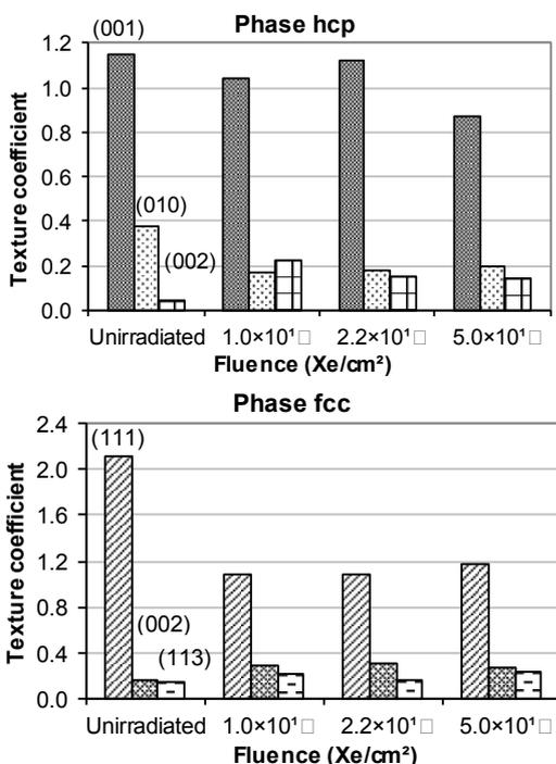
Fig. 7. Texture coefficients of titanium sample
