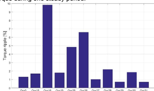
Fig. 8: Magnitude of torque ripple with variable rotor slit number
