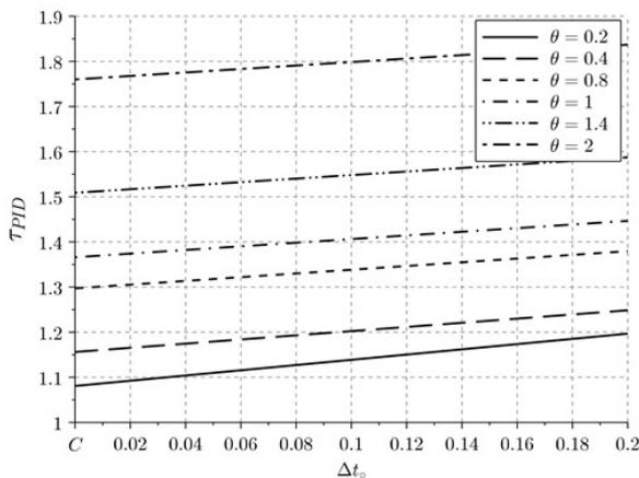
Fig. 4. Optimal settings of  $\tau_{PID} = f(\Delta t_o, \theta)$  according to (15)
