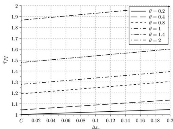
Fig. 6. Optimal settings of  $\tau_{PI} = f(\Delta t_o, \theta)$  according to (13)
