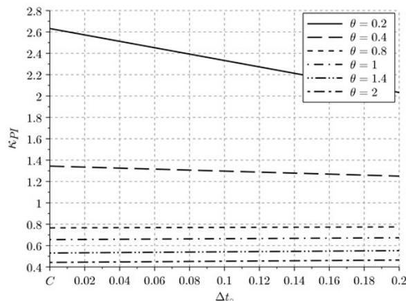
Fig. 5. Optimal settings  $\kappa_{PI} = f(\Delta t_o, \theta)$  according to (12)
