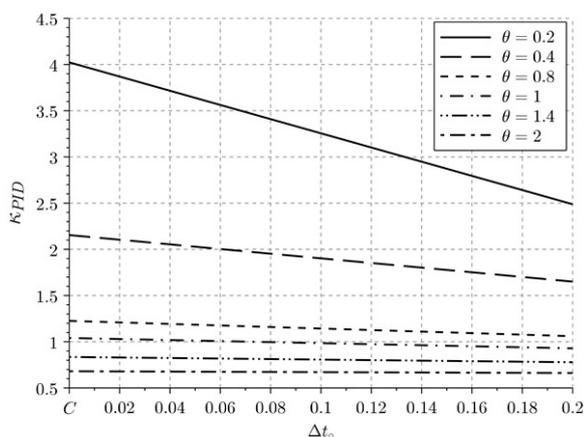
Fig. 3. Optimal settings  $\kappa_{PID} = f(\Delta t_o, \theta)$  according to (14)
