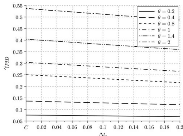
Fig. 7. Optimal settings  $\gamma_{PID} = f(\Delta t_o, \theta)$  according to (16)
