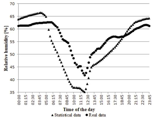
Fig. 8. Relative humidity values at height 0.1 m for statistical and real weather data
