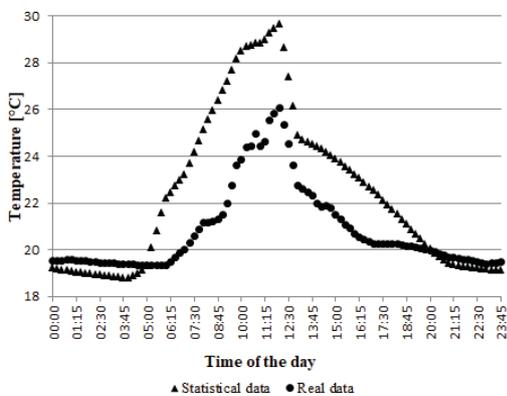
Fig. 6. Temperature values at height 1.1 m for statistical and real weather data
