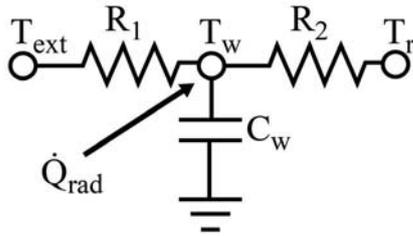
Fig. 2. 2R1C model of wall
