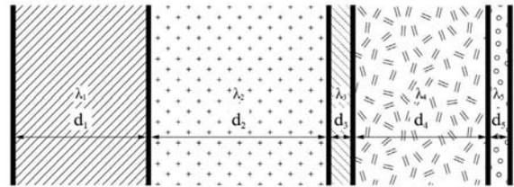
Fig. 3. Visualization of western wall ( $d$  – material thickness,  $\lambda$  – thermal conductivity of material)
