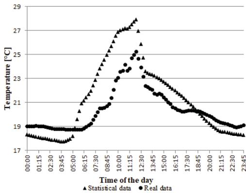
Fig. 5. Temperature values at height 0.8 m for statistical and real weather data
