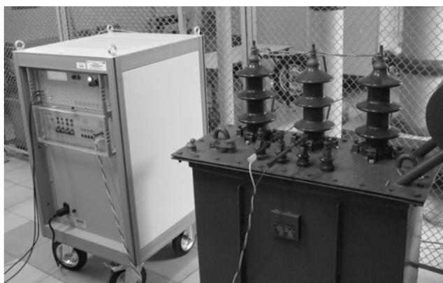
Fig.3. View of 3-phase 15 kV/0.4 kV distribution transformer and connected MIG0618SS surge generator.
