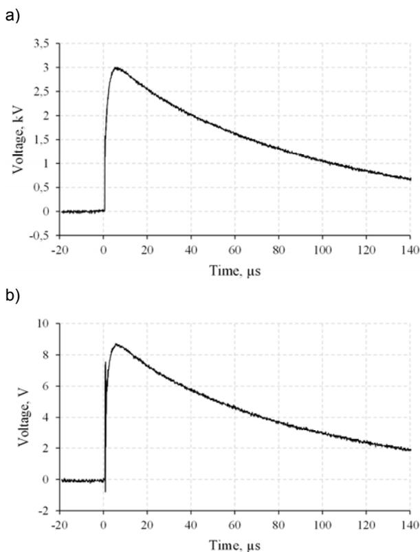
Fig.7. The voltage signals recorded during the test of antenna for one of configuration variant. a) surge voltage transient from MIG0618 generator. b) voltage waveform from one of antenna outputs at the end of 10 meter terminated coaxial cable.
