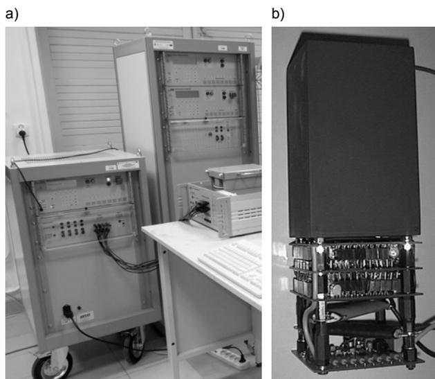
Fig.2. a) Generators: MIG0618SS (on the left) and MIG0600MS (on the right); b) High voltage module of MIG generator.
