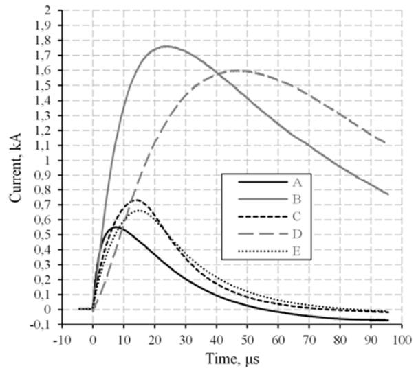
Fig.6. Comparison of current waveforms at injection point for different variants of the test setup.
