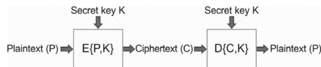
Fig. 2. The scheme of encryption (E) and decryption (D): Plaintext (message), Ciphertext (encrypted message)
