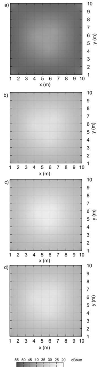
Fig. 6. Spatial distributions of the magnetic field magnitude in the horizontal plane  $z = 26$  m for geometries shown in Figs. 1 and 4 (the frequency is 25 kHz).
