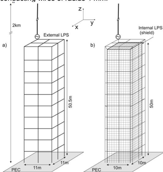
Fig. 1. Models of external LPS (a) and LPS integrated with internal wire-grid shield (b).
