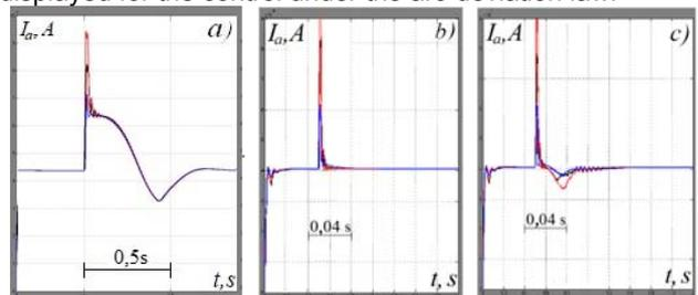
Fig. 6. Time dependencies of the current  $I_a(t)$  for regulating the symmetrical short circuit a) by the single-loop ACS with the high-speed circuit b) and by the double-loop ACS for EM control based on the current deviation
