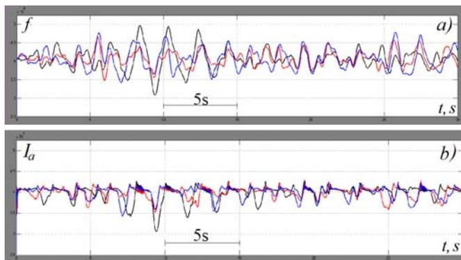
Fig. 9. Perturbations of the arc length  $f(t)$  in the phases a) arc currents  $I_a(t)$  b) when using the double-loop ACS at the end of the solid fusion mixture melting stage
