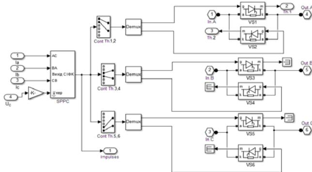
Fig. 4. Simulink model of one parallel TRG with the pulse-phase control system and power thyristors
