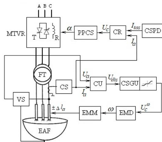
Fig. 1. Functional block diagram of the double-loop ACS for EM of the arc furnace
