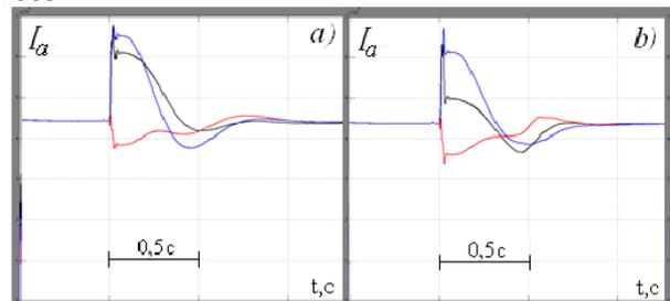
Fig.7. Time dependencies of arc currents for regulating the non-symmetrical short circuit in phase A by the double-loop ACS for different laws of arc length regulation and PI regulator of arc currents of the high-speed circuit
