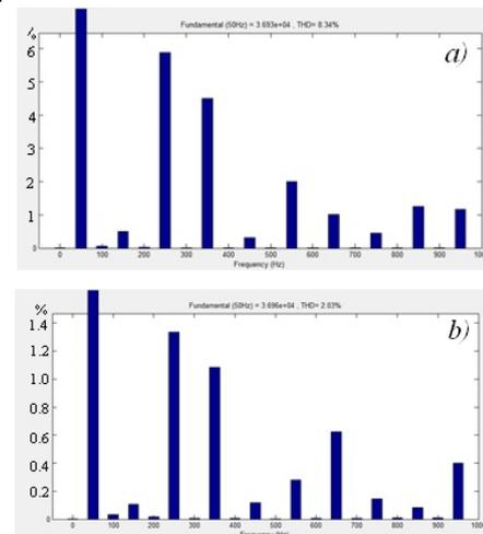
Fig.10. Amplitudes of the arc current harmonics for using one PTRG a) and three PTRG b) in MTRV for the differential control law
