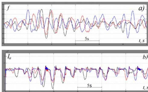
Fig. 8. Perturbations of the arc length  $f(t)$  in the phases a) and the respective arc currents  $I_a(t)$  b) of the double-loop ACS at the beginning of the solid fusion mixture melting stage
