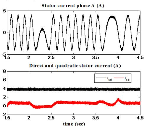
Fig.14 Stator currents of the induction motor with low speed region during speed reversal
