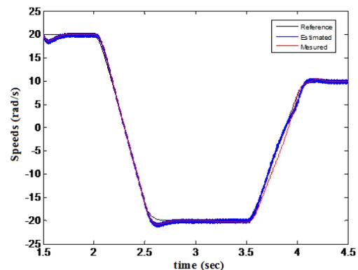
Fig.11 Performance of MRAS-Neural Self-Tuning IP observer with low speed region during speed reversal
