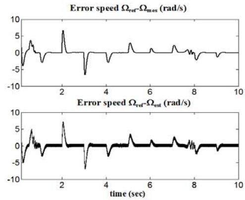
Fig.8 Speeds errors of the induction motor
