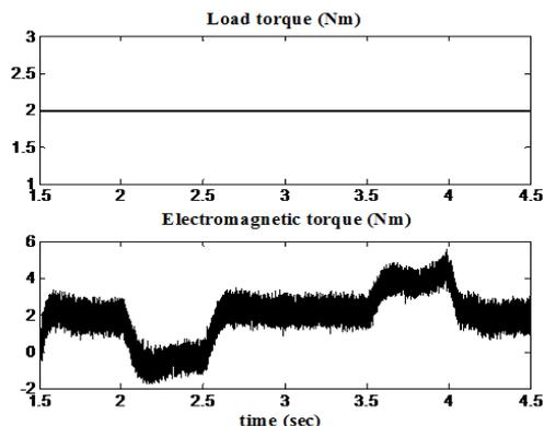
Fig.13 Electromagnetic torque of the induction motor with low speed region during speed reversal
