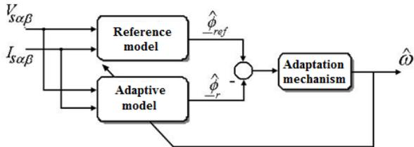
Fig.2.Structure of model reference adaptive systems
