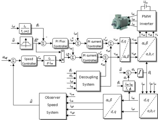
Fig.1.Direct field-oriented control for induction motor equipped with observer speed system
