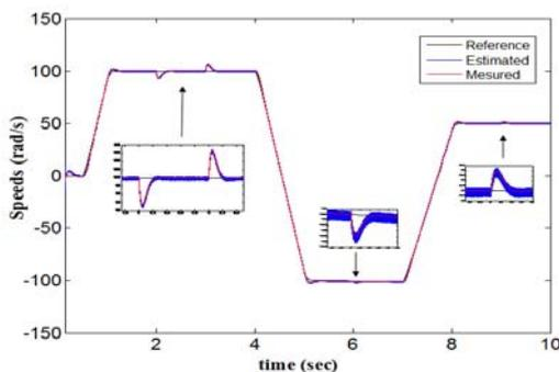
Fig.7 Performance of MRAS-Neural Self-Tuning IP observer with speed reverse and load charge change
