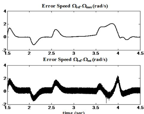
Fig.12 Speeds errors of the induction motor with low speed region during speed reversal
