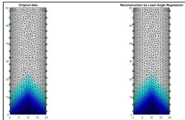
Fig. 2. The damp cellular concrete block and reconstruction based on the Least Angle Regression with 2 side measurements (2x16 electrodes) – models of moisture 2D.
