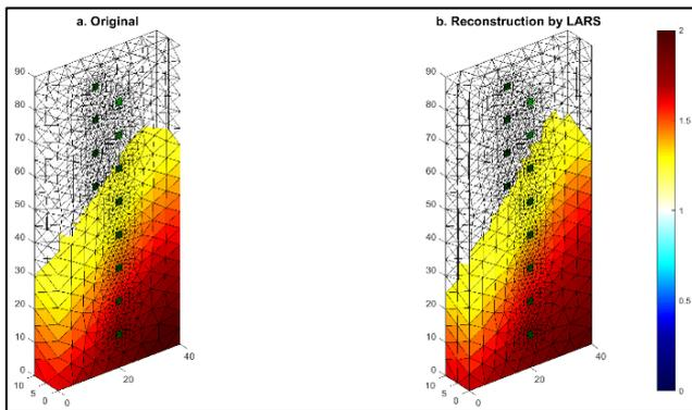
Fig. 4. The damp cellular concrete block and reconstruction based on the Least Angle Regression with 2 side measurements (2x8 electrodes) – models of moisture I.
