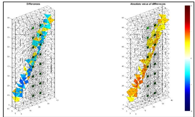
Fig. 5. The damp cellular concrete block and reconstruction based on the Least Angle Regression with 1 side measurements (2x8 electrodes)– model II.
