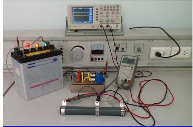
Fig. 6. A 100W prototype of a two level dual charge-pump DC-DC converter setup
