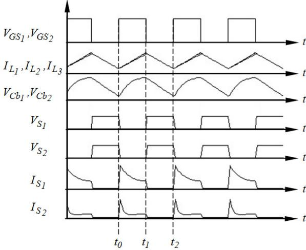
Fig. 2. Key waveforms of the proposed converter.
