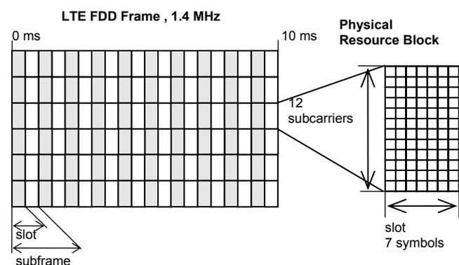
Fig.1. Structure of the frame in LTE, type 1 (FDD)
