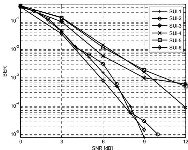
Fig.5. BER values determined using SUI models
