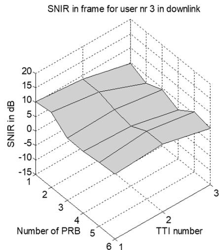
Fig.8. SNIR level for user 3 in the downlink versus number of PRB and TTI number, for frequency band 800/900 MHz, urban environment, and 3GPP channel model without fluctuations
