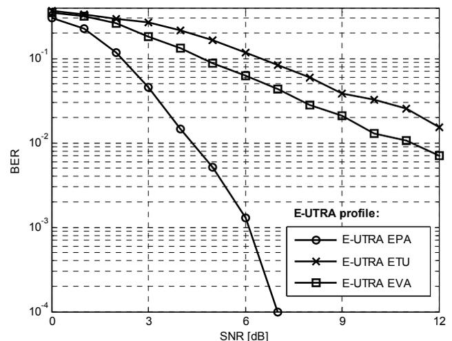
Fig.4. BER values for different profiles of E-UTRA model
