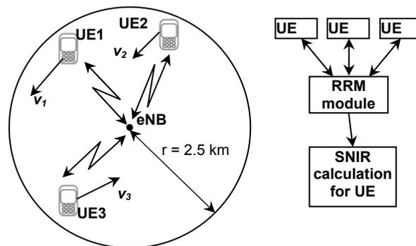
Fig.6. Block diagram of the network used for SNIR level calculation
