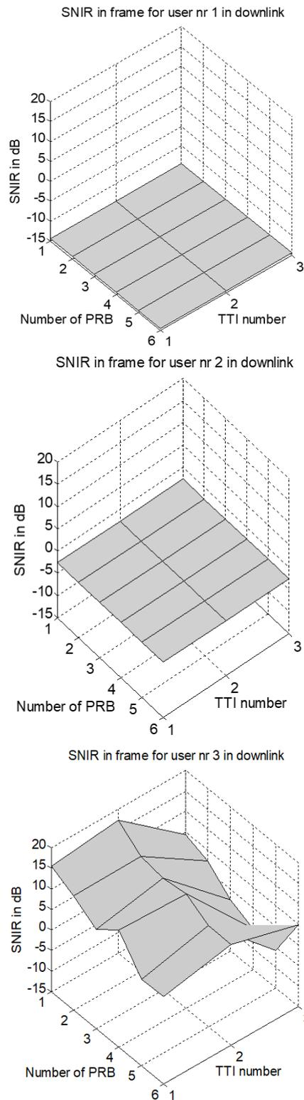
Fig.7. SNIR level for users in the downlink versus number of PRB and TTI number for frequency band 800/900 MHz, urban environment, and 3GPP multipath channel model with random fluctuations
