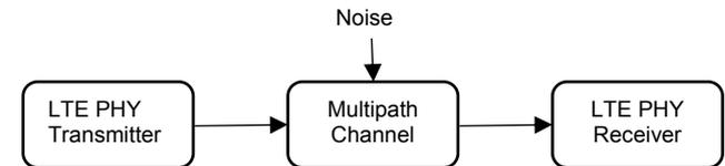
Fig.3. The block diagram of the simulation model
