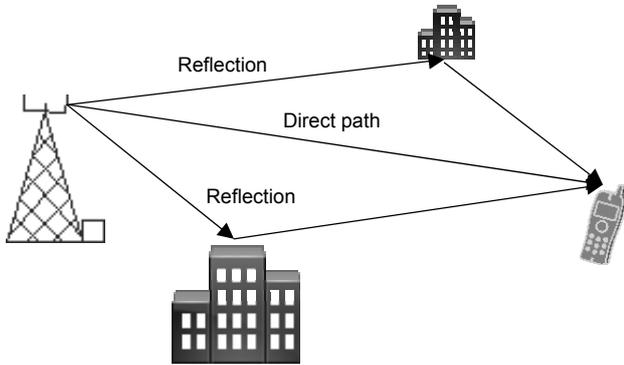
Fig.2. The example of a multipath propagation
