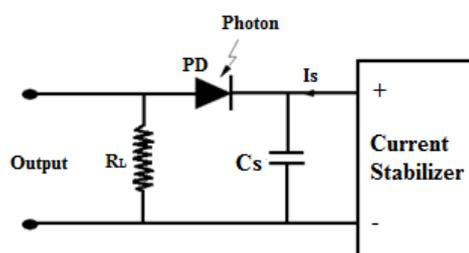
Fig. 1. Constant current temperature compensation.
