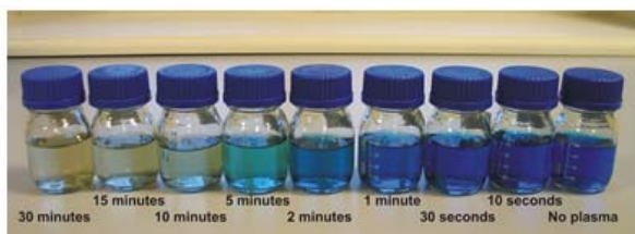
Fig. 6. Photograph of MB samples after plasma treatment. Initial concentration of MB and power dissipated during processing were equal to 20 mg/L and 23 W respectively.
