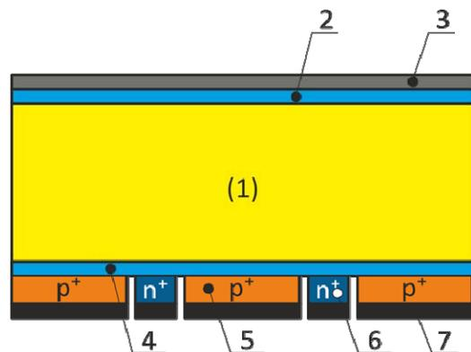
Fig.3. Schematic diagram of the tested HIT-IBC solar cell structure (sample 1): 1 – n-type silicon substrate, 2 – front passivation layer, 3 – anti-reflective coating, 4 – a-Si intrinsic thin layer, 5 – p<sup>+</sup> - type region, 6 – n<sup>+</sup> - type region, 7 – electrode
