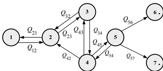
Fig.1. Oriented graph interpreting the set of conditions of electrical safety system at EHV electric installations and possible transitions between them
