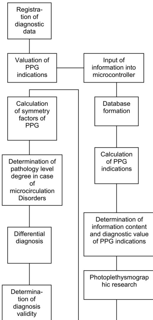
Fig.3 Algorithm of photoplethysmo-graphic data processing for diagnosis of cardiovascular system diseases
