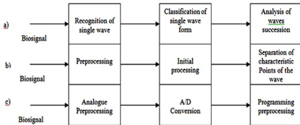
Fig.2. On-line processing of biological signals: a) general scheme; b) conveyer for recognition of a single wave; c) block-diagram of preliminary processing of biosignal
