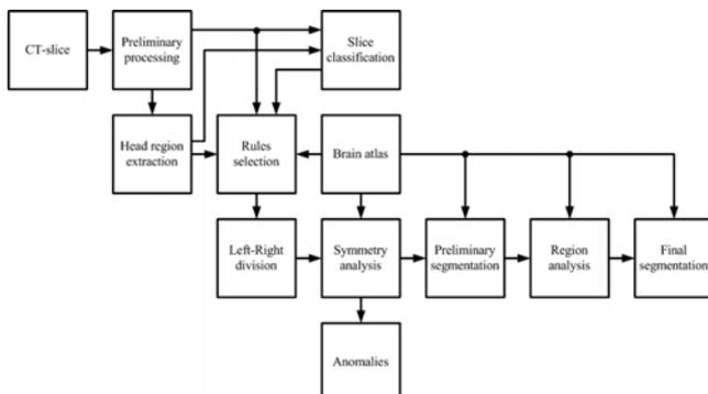
Fig.2. The main stages of the input slice processing
