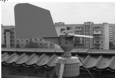
Fig.1. Burkard Spore Trap on the roof of the Chemistry Building of the Vinnytsia National Pirogov Memorial Medical University
