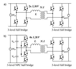
Fig. 5. Dual Active Bridge with multilevel converter on MV side
