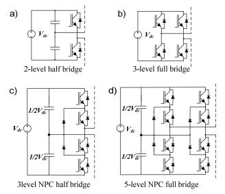
Fig. 3. Module topologies: a) half-bridge – 2-level, b) full-bridge – 3-level, c) NPC half-bridge – 3-level, d) NPC full bridge – 5-level
