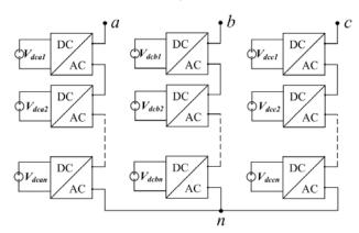
Fig. 2. Block scheme of three-phase Modular Multilevel Converter [9], [10]
