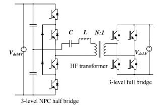
Fig. 6. Series resonant converter with multilevel module on MV side
