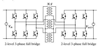
Fig. 7. Three-phase Dual Active Bridge
