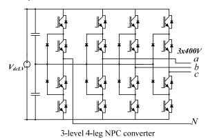
Fig. 9. Three-level four-leg topology proposed for LVC
