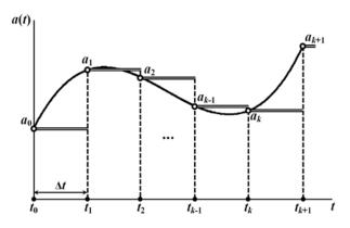
Fig.1. The sequence the reading of vibration acceleration values a (*t*)
