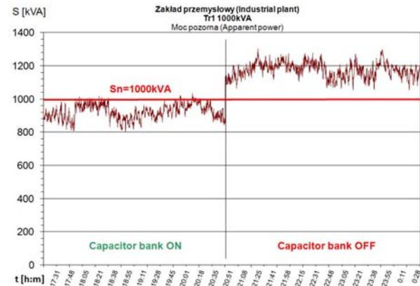
Fig. 3. Apparent power graph with a reactive power compensation unit correspondingly off and on
