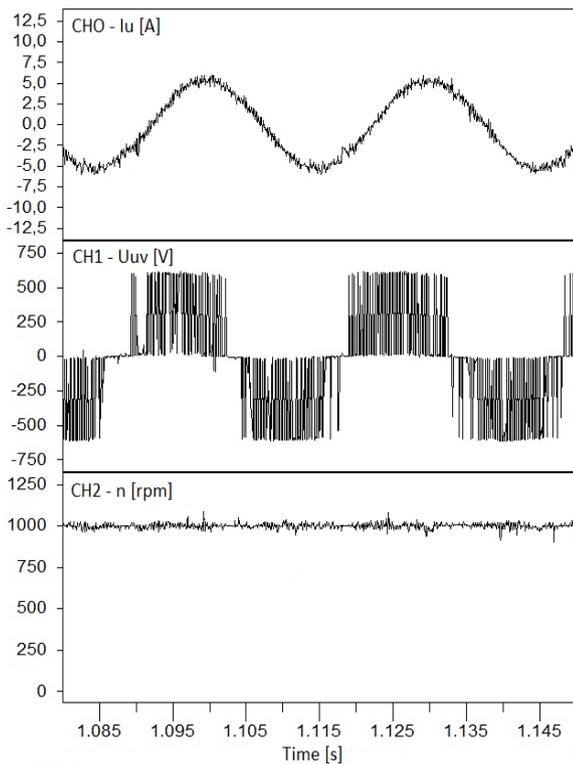
Fig. 4. Time characteristics of the phase current, phase-to-phase voltage and rotational speed for steady-state conditions
