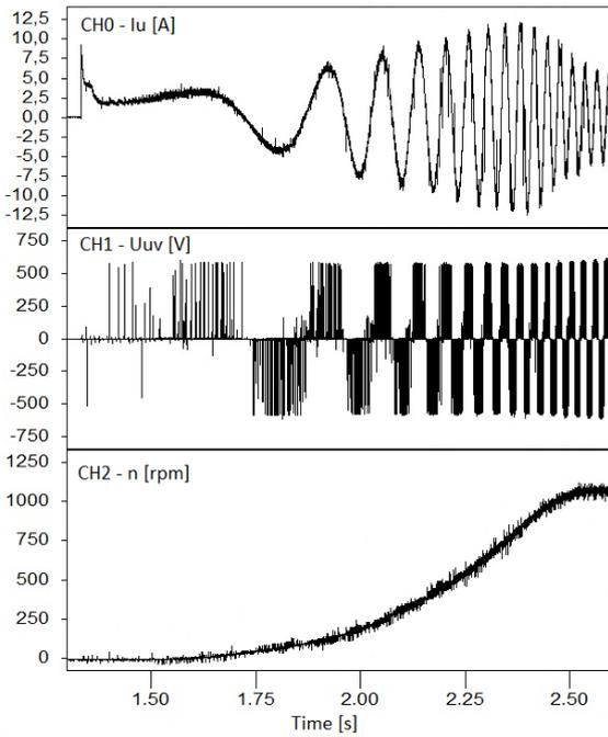
Fig. 3. Time characteristics of the phase current, phase-to-phase voltage and rotational speed at start-up
