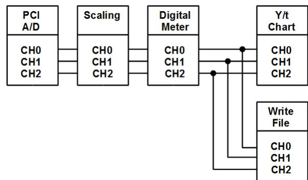
Fig. 2. Block diagram of the system for registering and visualising the time curves of voltage, current and rotational speed of the AC drive
