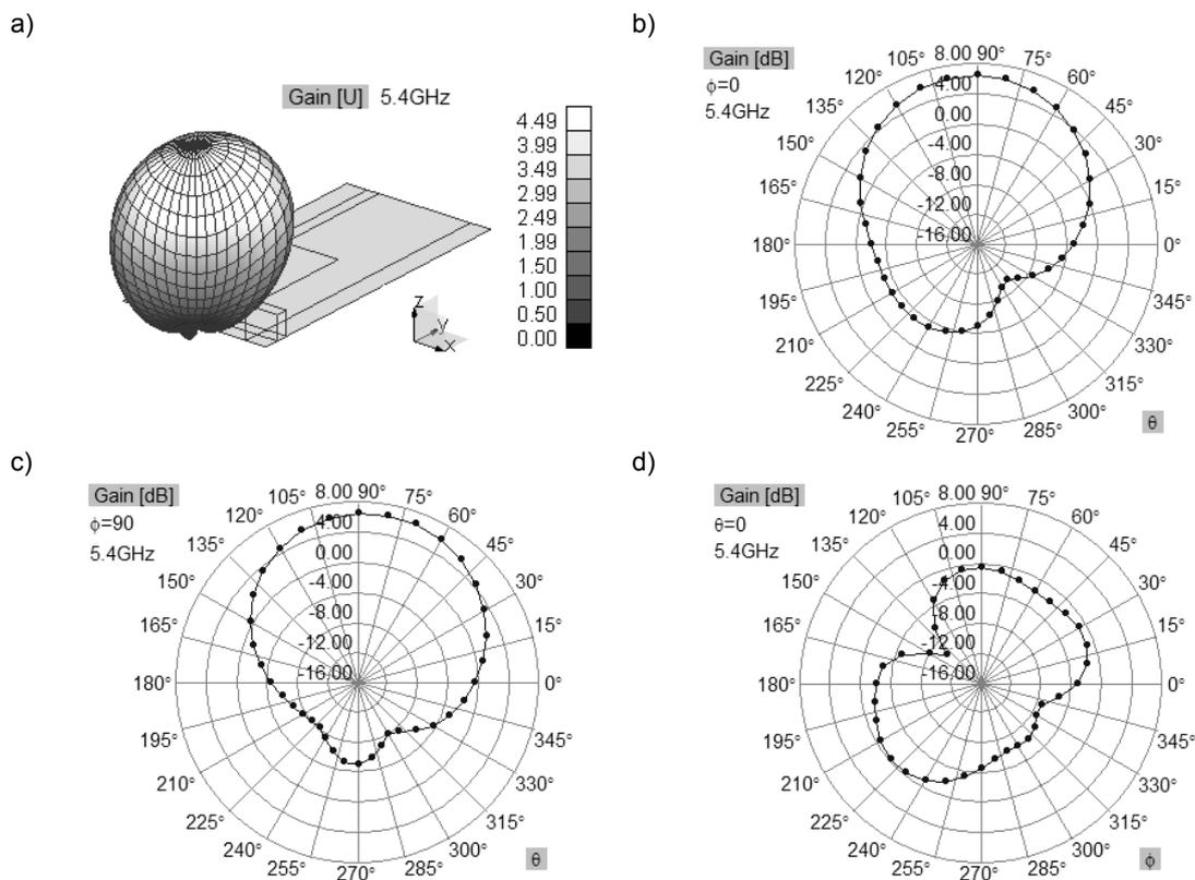
Fig.4. 3D radiation pattern of the antenna at 5 GHz operation band in a linear scale (a) and the main cross-sections of radiation patterns of the antenna: x-z plane (b), y-z plane (c) and x-y plane (d)
