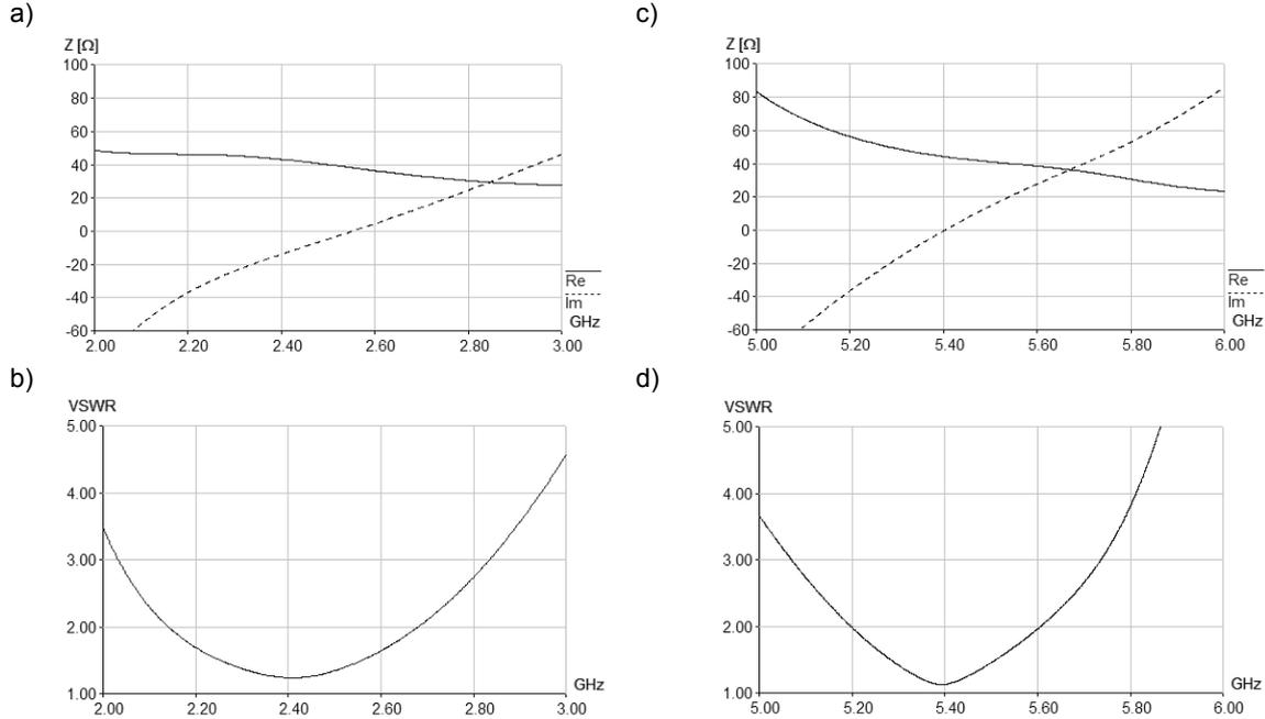
Fig.2. Frequency characteristics of the antenna impedance in lower 2,4 GHz (a) and upper 5 GHz (c) frequency band and corresponding characteristics of voltage SWR of the analyzed antenna (b,d)
