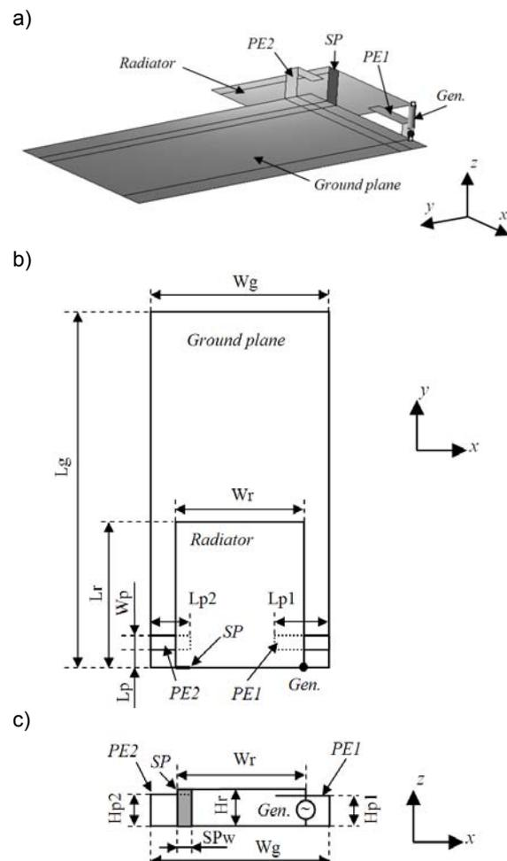
Fig.1. The structure of the analyzed antenna: an overall view from the bottom of the antenna (a) and the projection on x-y plane (b) and x-z plane (c)
