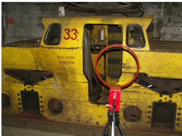
Fig. 2. Traction locomotive, loop antenna for magnetic field measurements in front
