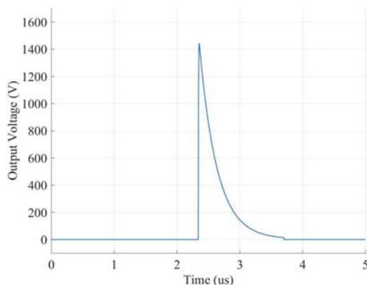
Fig. 2. Simulated output voltage waveform of the HVPG
