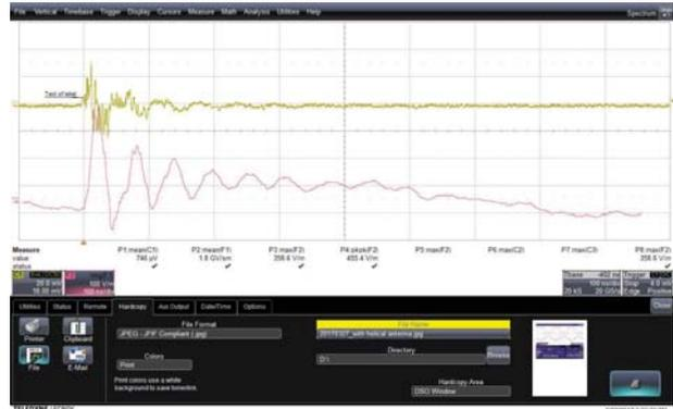
Fig. 8. The electrical field measured using free field D-Dot probe
