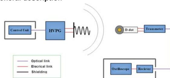
Fig. 1. Schema describing the general structure of the test-bench
