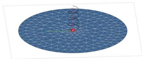
Fig. 4. 3D model of helical antenna using FEKO software
