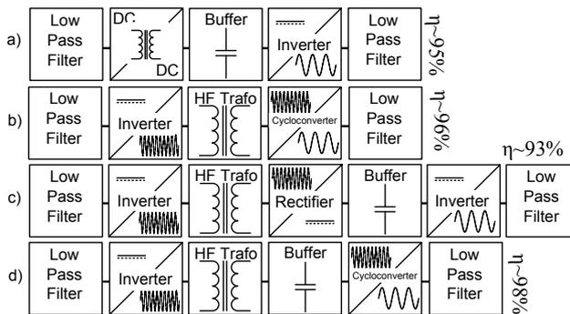
Fig. 8. Different variants of inverters topology for PV installations with HF transformers
