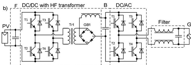
Fig. 6. An example of topology with HF transformer that is on the market, where: F - Low Pass Filter, B - Buffer, G - power grid, PV - photovoltaic panels, HF - high frequency
