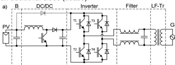
Fig. 4. An example of topologies with LF transformer that are on the market, where: B - Buffer, G - power grid, LF-Tr Low frequency transformer, PV - photovoltaic panels
