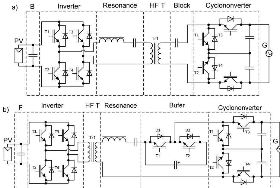
Fig. 9. An example of topologies with cycloconverter instead of AC/DC and DC/AC converters: without buffer (a) [7] and with a buffer (b) [1], where: F - Low Pass Filter, G - power grid, PV - photovoltaic panels, HF T - high frequency transformer, B - Buffer
