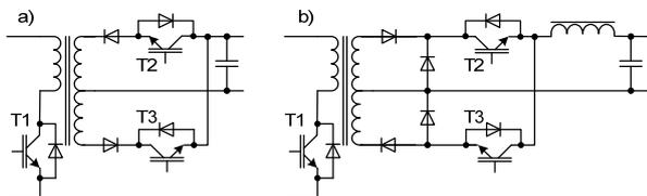
Fig. 7. a) Example of inverters based on Flyback (a), and Forward converter (b).
