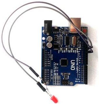
Fig.1. Arduino/Genuino board with connected LED
