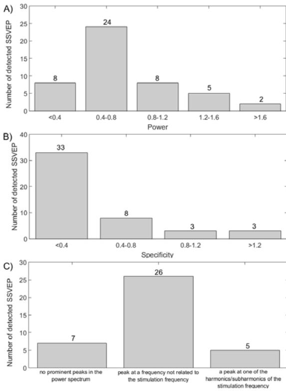
Fig.4. The summary of the analysis of all 85 power spectra; a) The distribution of power of correctly detected SSVEPs; b) The distribution of specificity of correctly detected SSVEPs; c) The structure of "non SSVEP detection" cases.
