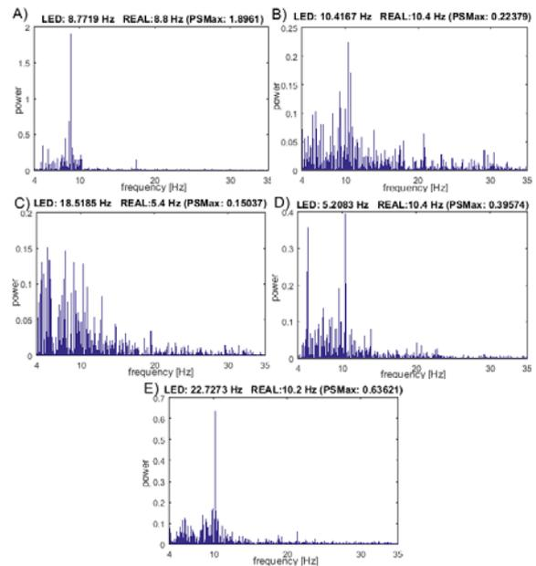
Fig.5. Different types of power spectra: a) SSVEP of a high specificity; b) SSVEP of a low specificity; c) no prominent peaks; d) a peak at a harmonic frequency e) a peak at a frequency not related to the stimulation frequency (peak at 10.2 Hz; stimulation frequency 22.73Hz).
