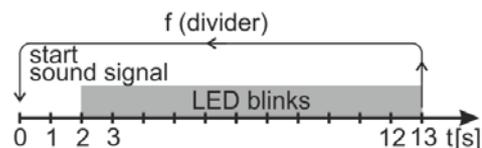
Fig.3. Timing scheme of the experiment. The trial starts with a sound signal intended to draw user attention. After 2 seconds LED starts to blink with a frequency  $f(divider)$ , where  $divider = 16$  [31.25Hz] and 100 [5Hz]. The EEG signal is recorded from the 4th to the 13th second of the trial. The same scheme is repeated for all 85 analyzed frequencies.
