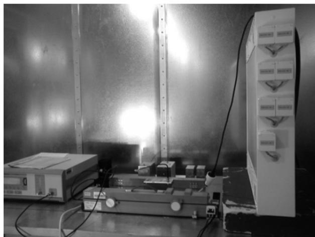
Fig. 7. The KNX model during the immunity to conducted disturbances test.
