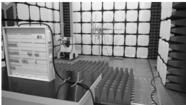
Fig. 5. The KNX model during the immunity test to radiated electromagnetic field.
