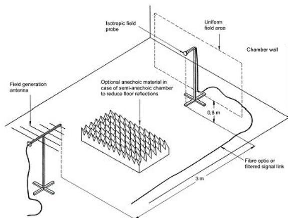
Fig. 4. Immunity to radiated electromagnetic field test setup [4].
