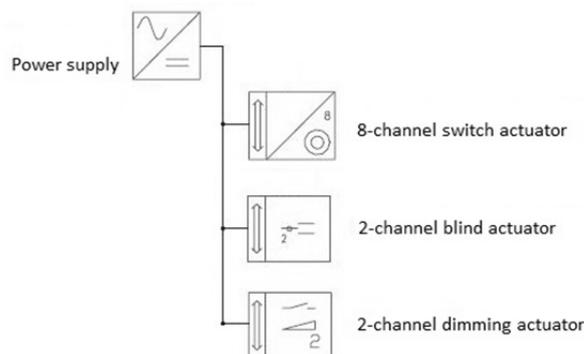
Fig. 3. Schema of connection of KNX elements [7].
