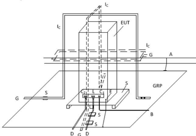
Fig. 8. Immunity to the power frequency electromagnetic field test setup, where: GRP- reference ground, A- protective grounding, S- insulated factor, EUT- device under test,  $I_c$ - inductive coil, E- protective clamp,  $C_1$ - power supply circuit,  $C_2$ - signal circuit, L- communication line, B- to power supply, D- to supply source, G- to the testing generator [9]
