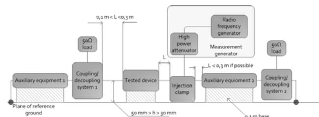
Fig. 6. System diagram of test setup for the immunity to conducted disturbances test [8].
