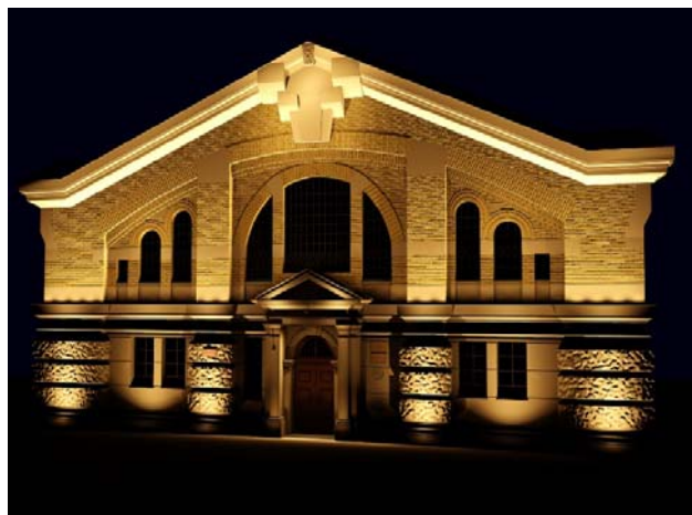
Fig. 3. Computer visualisation of concept of floodlighting of the Old Boiler Room Building (angle 0°).
