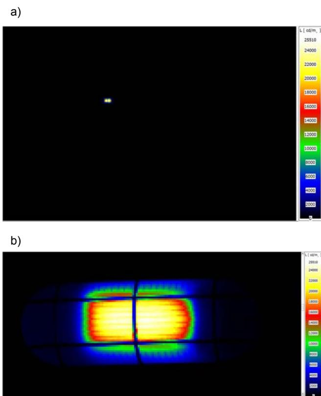
Fig. 4. a) The map of luminance determined by LMK photometer in laboratory, b) enlarged fragment containing the source of glare. The maximum luminance of the source 25 510 cd/m<sup>2</sup>
