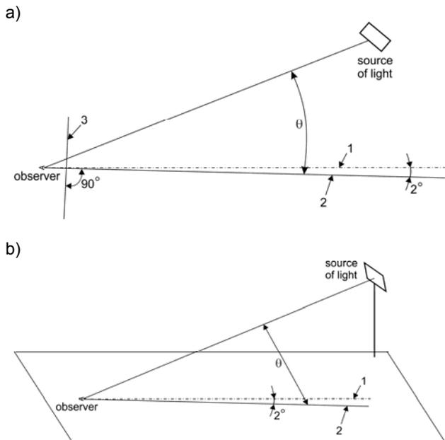
Fig.1. Definition of the angle  $\theta$ : 1 – the horizontal line, 2 – the line of sight ( $2^\circ$  below the horizontal line), 3 – the plane of  $E_{eye}$  perpendicular to the line of sight, a) the cross section of the field of view [2], b) the spatial arrangement [7]
