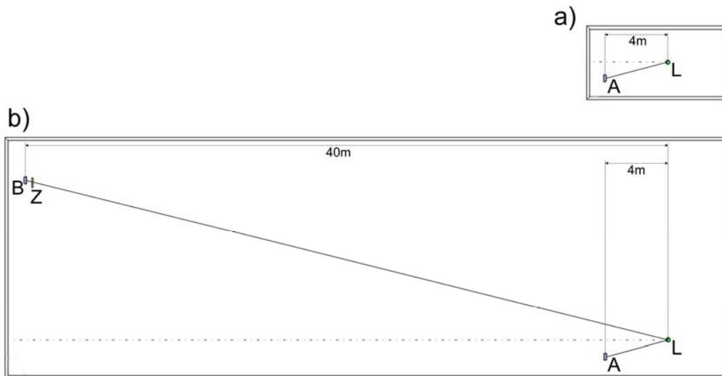
Fig. 3. The arrangement of: light sources (**A** and **B**), the opaque shield (**Z**) and the LMK photometer (**L**). In the experiment and simulations we used: a) in the laboratory: L + A, b) in DIALux simulation: Case 1: L + A, Case 2: L + A + B, Case 3: L + A + B + Z.
