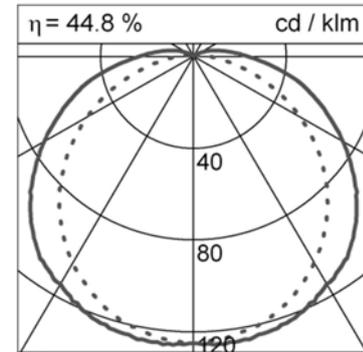
Fig. 2. The curves of luminous intensity for fluorescent luminaire with frosted and textured glass diffuser, used in experimental studies [15]
