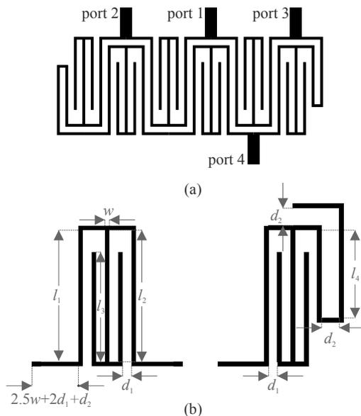
Fig. 1. (a) Layout of the example compact RRC [2]; (b) Parameterized layouts of shunt-stub-based TLs
