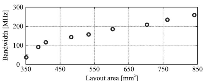
Fig. 3. Pareto-optimal set representing the best possible trade-offs between bandwidth and layout area of the compact RRC, acquired by means of the presented multi-objective optimization procedure
