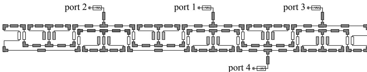
Fig. 2. Equivalent circuit model of the example compact RRC, implemented in Agilent ADS [8]. Highlighted components have different sets of implicit space mapping parameters  $p$  assigned to them (dark grey:  $\epsilon_1, h_1$ ; grey:  $\epsilon_2, h_2$ ; white:  $\epsilon_3, h_3$ )
