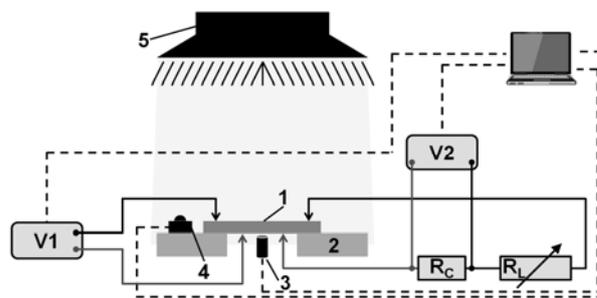
Fig.2. Schematic diagram of the laboratory stand: 1 – solar cell, 2 – supporting construction, 3 – temperature sensor, 4 – pyranometer, 5 – light source, V1 – Fluke 289, V2 – Hameg HMC8012,  $R_C$  – shunt resistor,  $R_L$  – adjustable load
