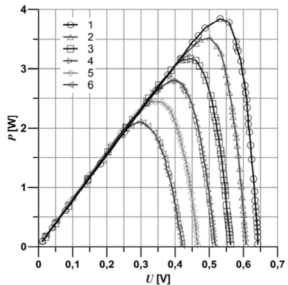
Fig.5. P-V characteristics of c-Si solar cell recorded at the irradiance  $E = 1000$  W/m<sup>2</sup> for different operating temperatures: 1 – -20°C, 2 – 0°C, 3 – 25°C, 4 – 50°C, 5 – 75°C, 6 – 100°C
