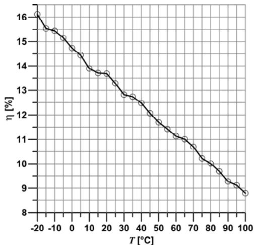
Fig.6. Efficiency of c-Si solar cell vs. operating temperature, recorded at the irradiance  $E = 1000 \text{ W/m}^2$
