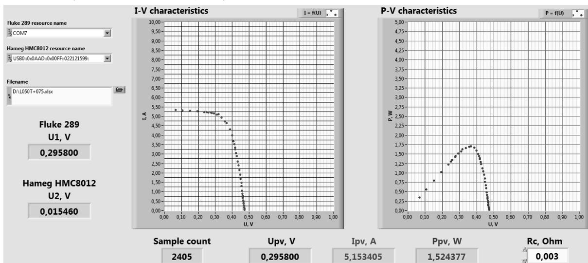
Fig.3. The main window of the PV Cells Meter software
