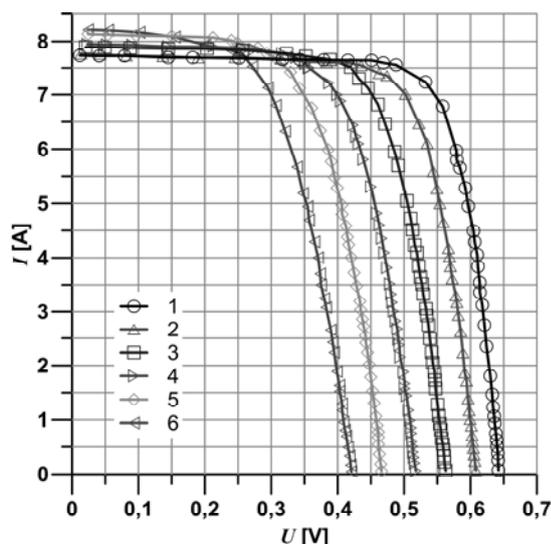
Fig.4. I-V characteristics of c-Si solar cell recorded at the irradiance  $E = 1000$  W/m<sup>2</sup> for different operating temperatures: 1 – -20°C, 2 – 0°C, 3 – 25°C, 4 – 50°C, 5 – 75°C, 6 – 100°C
