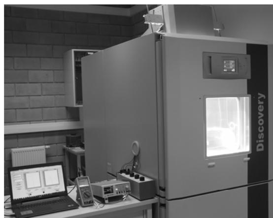
Fig.1. Photograph of the laboratory stand for investigating the influence of environmental conditions on electrical parameters of PV cells
