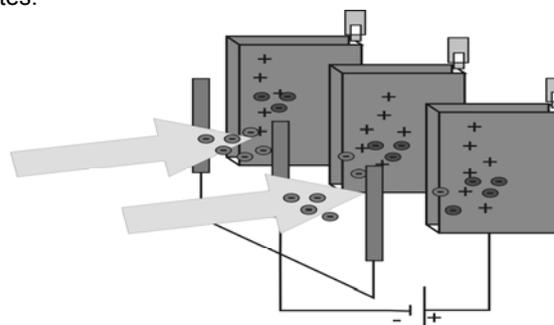
Fig.1. Conceptual diagram of an electrostatic precipitator
