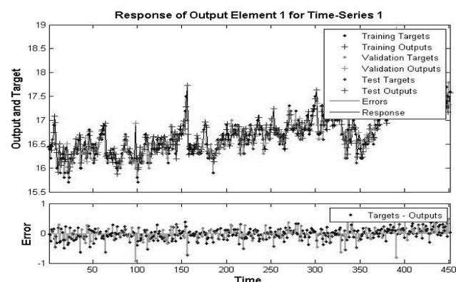
Fig.6. ESP NNARX model response plot
