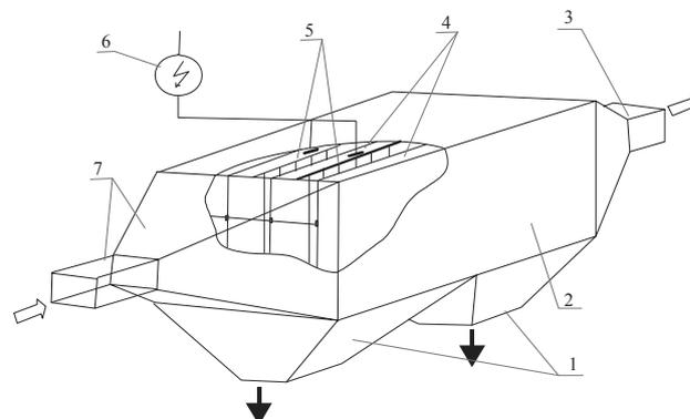
Fig.2. Scheme of horizontal, two stage electrostatic precipitator (ESP): 1 - bulk hopper, 2 - particulator chamber, 3 - confuser and outlet channels, 4 - collecting electrodes system, 5 - corona electrode system, 6 - high voltage supply.
