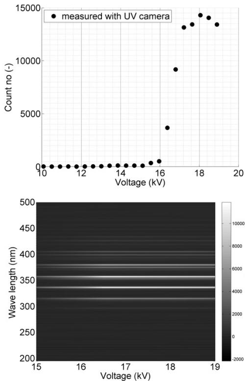
Fig. 2. Optical signals registered with the two considered methods on the cylindrical insulator
