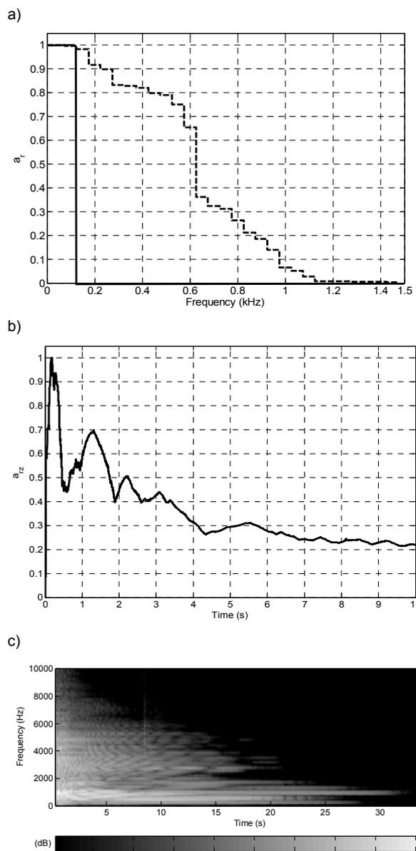
Fig.2. Changes of normalized spectral power density of tested transformer (a): continuous line – ideal case, dashed line – tested unit, (b) oscillations of the envelope of the transient vibrations signal, (c) spectrogram of transient vibrations signal
