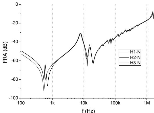
Fig.1. FRA results of transformer TORc 16000/115
