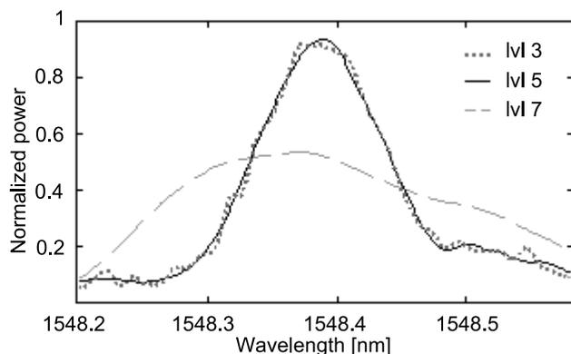
Fig. 4. Denoised spectrum with different decomposition levels
