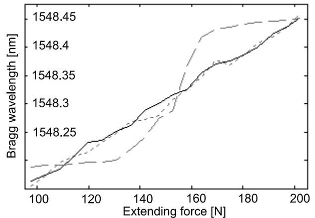
Fig. 5. Force to wavelength shift processing characteristics traced from spectra denoised with different decomposition levels
