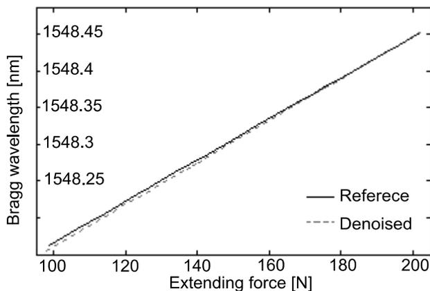
Fig. 6. Linear models of reference and calculated sensor processing characteristics
