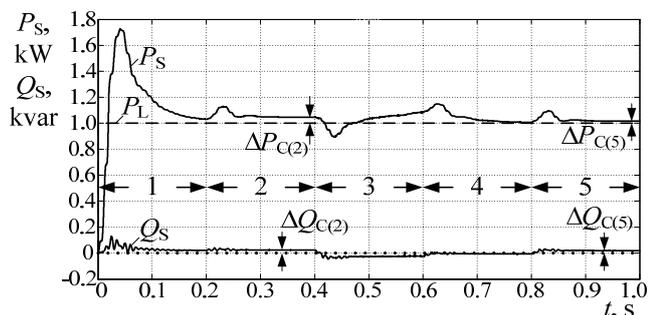
Fig. 11. Waveform of active power  $P_S$  and reactive power  $Q_S$  of source in states 1÷5
