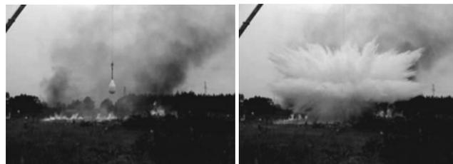
Fig. 1. On the left side of the figure: the water bomb filled with water and cylindrical explosion material, on the right: production of the water aerosol
