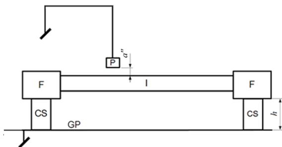
Fig. 2. Potential distribution measurement system. I – insulator; F-fittings; P – voltage probe (Trek 520); CS – conducting support; GP - grounded plate, distances:  $a'' = 7$  mm,  $h = 20$  mm
