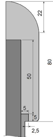
Fig. 9. Details of the fitting used in simulation
