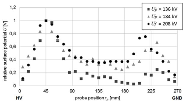
Fig. 6. Relative (related to the maximum value) surface potential distributions measured after applying positive impulse voltage with ( $U_f$ ) and without ( $U_p$ ) flashover occurrence. HV and GND refer to high voltage and grounded fittings respectively. Model: B-HTV
