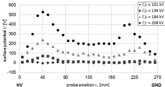
Fig. 5. Surface potential distributions measured after applying positive impulse voltage with ( $U_f$ ) and without ( $U_p$ ) flashover occurrence. HV and GND refer to high voltage and grounded fittings respectively. Model: B-HTV
