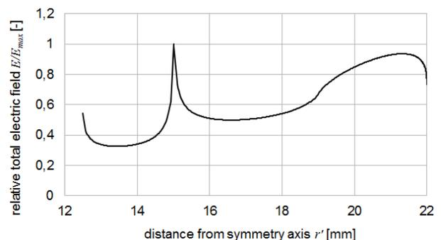
Fig. 11. Electric field (modulus value) distribution on line A (see Fig. 10).
