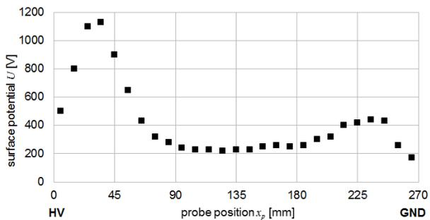
Fig. 3. Surface potential distribution measured after positive impulse flashover ( $U_f = +201.5$  kV). HV and GND refer to high voltage and grounded fittings respectively. Model: EG-LSR
