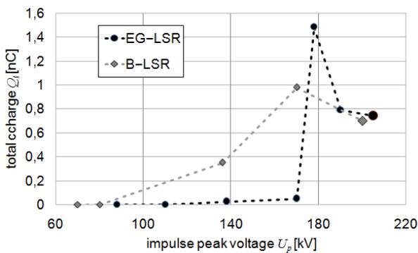
Fig. 8. Total charge as a function of impulse voltage  $U_p$ . Points for highest voltages - for flashover.
