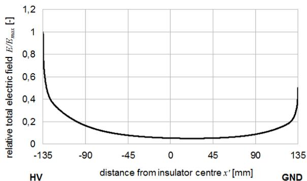
Fig. 12. Electric field (modulus value) distribution between fittings edges (sharpest part). HV – upper (high voltage) fitting, GND – bottom (grounded) fitting.
