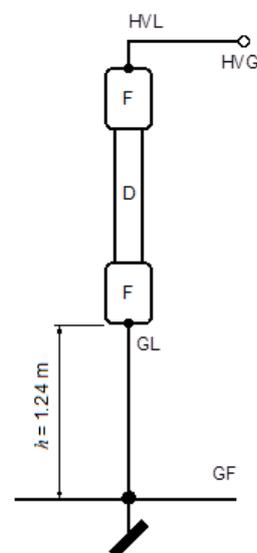
Fig. 1. Simplified scheme of insulator attachment. Symbols: GF – grounded floor, GL – grounding line, HVL – high voltage line, HVG – connection to high voltage generator. Not scaled
