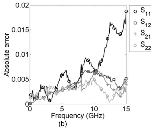
Fig. 6. Modeling results of the device no. 1 at the “cold pinch-off” condition  $U_{DS}=0\text{ V}$ ,  $U_{GS}=-5\text{ V}$ . (a) – model fitting results – markers denotes modeled values and solid lines measurement results; (b) – absolute error between the model and the measurement results as a function of frequency
