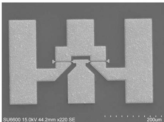
Fig. 1. SEM picture of GaN HEMT device manufactured by ITME
