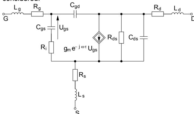
Fig. 5. GaN FET small-signal equivalent circuit
