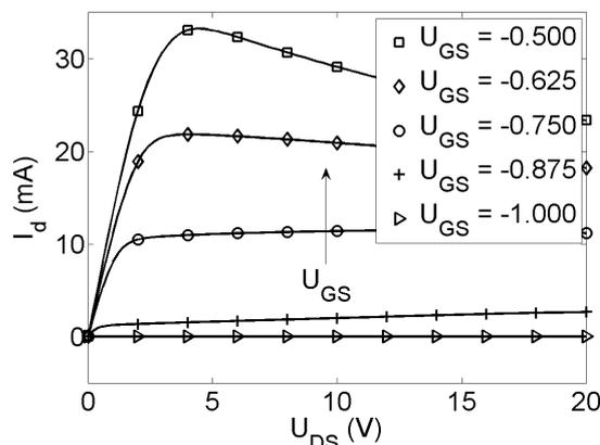
Fig. 2. Drain current as the function of the drain voltage  $U_{DS}$  for different gate voltages swept from -1 to -0.5 V with 0.125 V step
