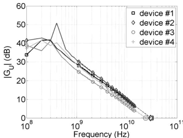
Fig. 4. Unilateral gain of the devices as the function of the frequency for the bias point:  $U_{ds} = 5$  V,  $I_{ds} = 20$  mA. Dashed line denotes linear extrapolation used to determine maximum oscillation frequency  $f_{max}$
