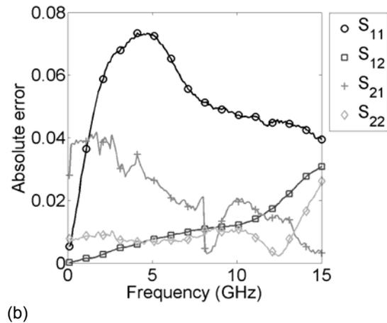
Fig. 7. Modeling results of the device no. 1 at the „hot” condition  $U_{ds}=5\text{ V}$ ,  $I_{ds}=20\text{ mA}$ . (a) – model fitting results – markers denotes modeled values and solid lines measurement results; (b) – absolute error between the model and the measurement results as a function of frequency
