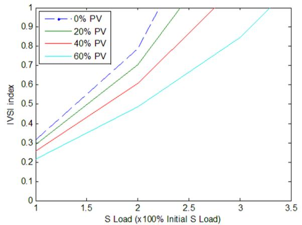
Fig.7. IVSI at Bus 61 with various PV penetration level
