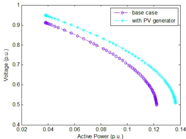
Fig.4. P-V curve of Bus 61 with integrated PV generator
