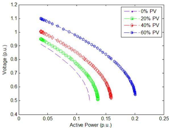
Fig.6. P-V curve of Bus 61 with various PV penetration level
