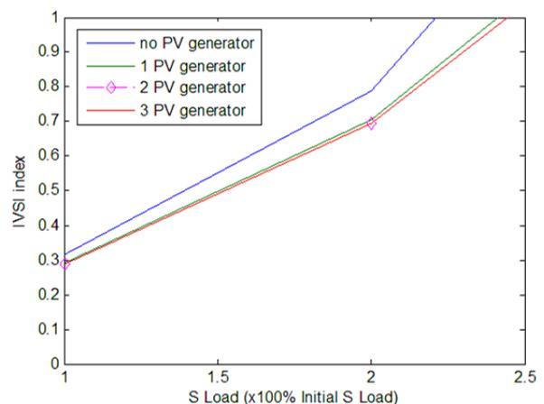
Fig.8. IVSI at Bus 61 (reference bus) with multiple PV generator
