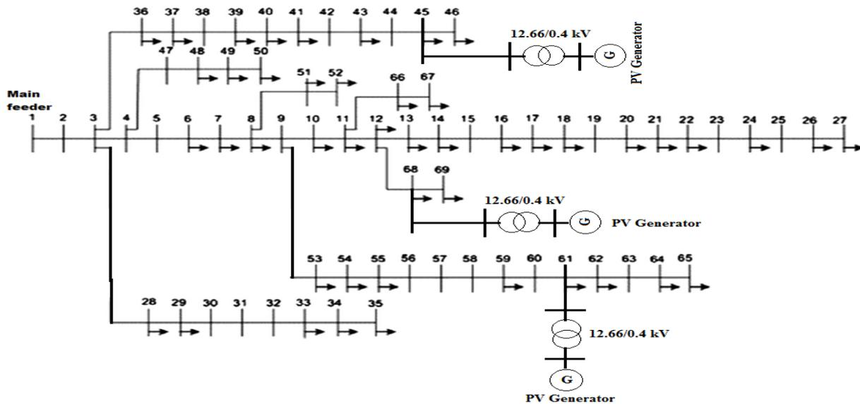
Fig.2. IEEE 69 radial distribution system with grid-connected PV generator
