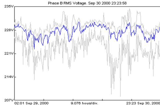
Fig. 10. Example of rms voltage fluctuation
