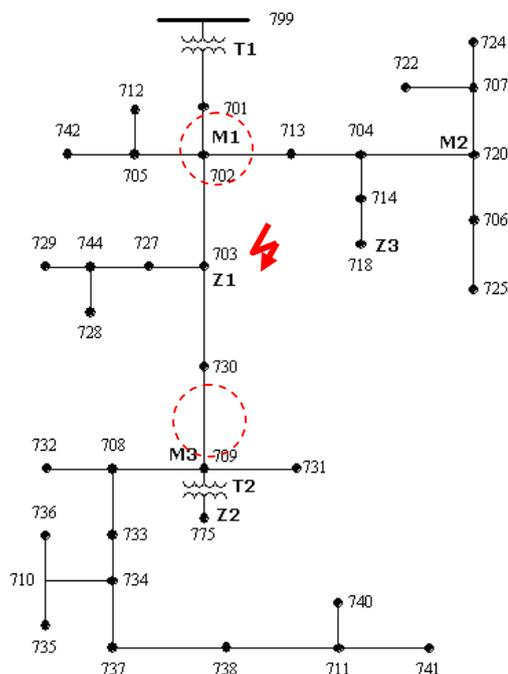
Fig. 12. Supply network model used to investigate the power flow during a short-circuit
