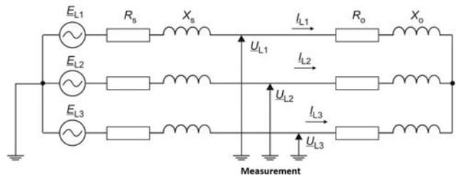
Fig. 7. Circuit diagram for asymmetry source location and identification
