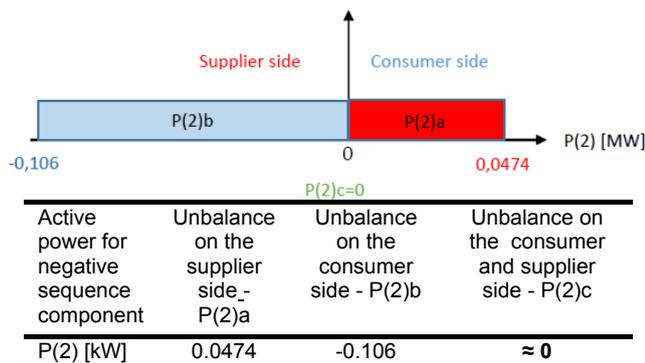
Fig. 9. TEST 2: Symmetrical voltages in PCC - the various components of the active powers for negative sequence component corresponding to the individual consumer and supplier emission levels
