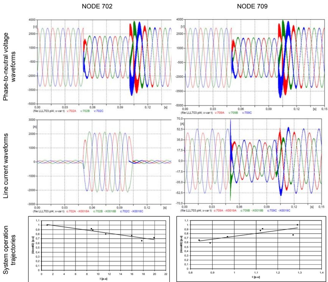
Fig. 13. Example results of a three-phase short circuit simulation in node 703 of 23 network model; waveforms of voltages and currents in nodes 702 and 709 (Fig. 13) as well as system operation trajectories in these points for phase L1 (analogous waveforms in other phases)
