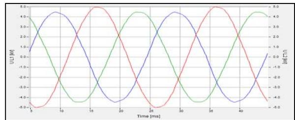
Fig. 6. Waveforms of asymmetrical voltages measured at PCC
