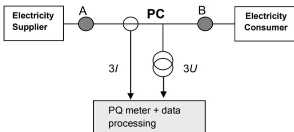
Fig. 1. Problem of locating the voltage disturbance sources
