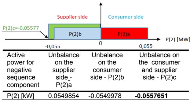
Fig. 8. TEST 1: Voltage asymmetry in PCC - equality under the active powers for negative sequence component corresponding to the individual consumer and supplier emission levels
