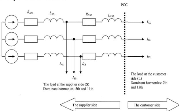
Fig. 3. Model of the electric power network chosen for simulations illustrating the active power flow method
