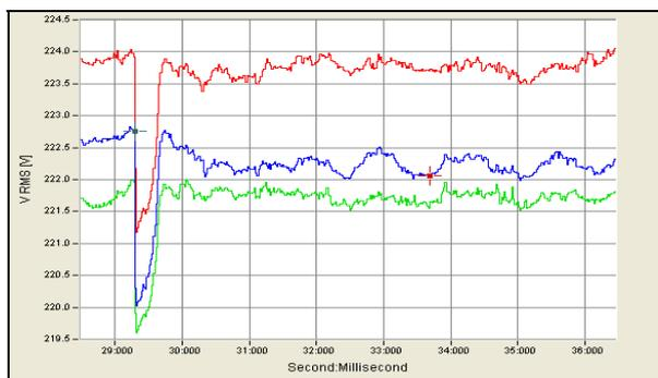
Fig. 11. Three-phase voltage dip
