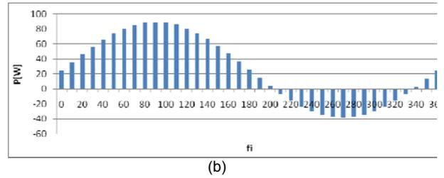
Fig. 5. Variation of the 5th harmonic active power at PCC for different values of the phase shift angle  $\varphi$  between the customer and supplier current and various relations between their rms values: (a) 1:1.2; (b) 1:1.8
