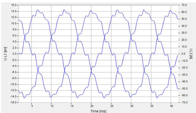
Fig. 2. Waveforms of distorted voltages measured at PCC
