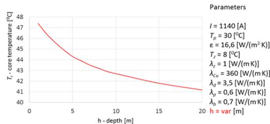
Fig. 4 Dependence of cable core temperature  $T_r$  on the system's distance  $h$  from the ground surface.
