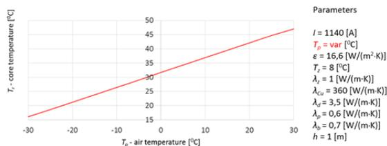
Fig. 5 Chart of three phase system cable core temperature  $T_r$  as dependent of air temperature  $T_p$ .
