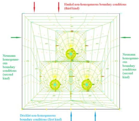
Fig.2 Three-phase high-voltage cable system laid in a concrete block under the ground surface with marked boundary conditions.
