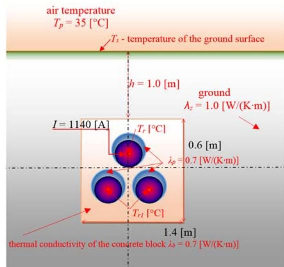
Fig.1 Three-phase high-voltage cable system of 110kV laid in a concrete block
