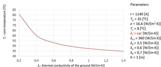
Fig. 6 Chart of three phase system cable core temperature  $T_r$  as dependent on thermal conductivity of the ground.
