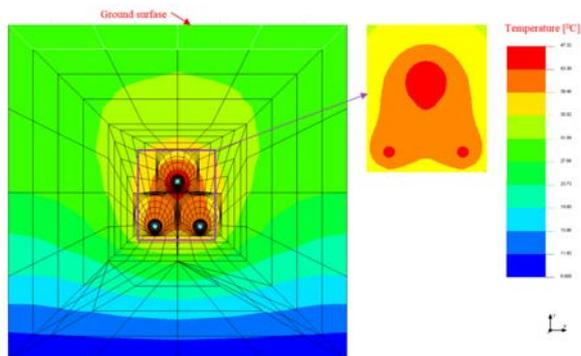
Fig. 3 Temperature field distribution of the three-phase system ( $h = 1\text{m}$ ).
