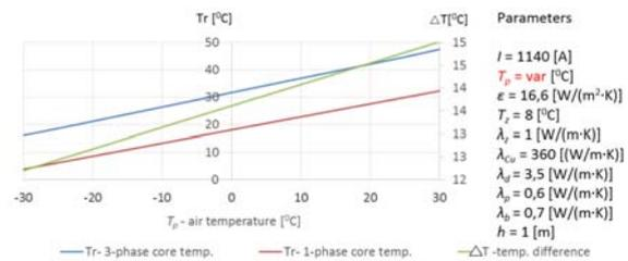
Fig. 18. Temperatures of the three phase cable core and single cable core and their temperature difference accounting for the changes of air temperature above the ground surface.
