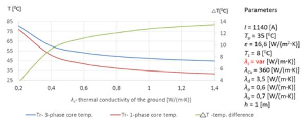
Fig. 19. Temperatures of the three phase cable core and single cable core and their temperature difference depending on thermal conductivity of the ground.
