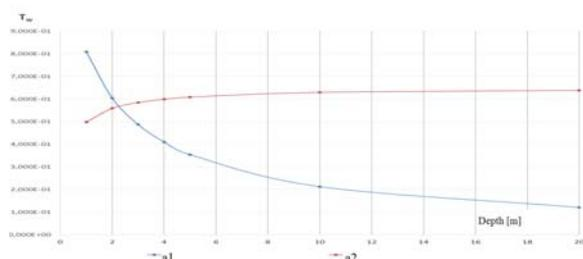
Fig. 14 Dependence of relative changes of cable core temperature  $T_w$  in the function of the cable system's distance from the ground surface for two parameters  $T_p$  and  $\lambda_z$ . The intersection point of the two curves defines the depth  $h = 2.2m$  at which the exchange of set elements occurs.
