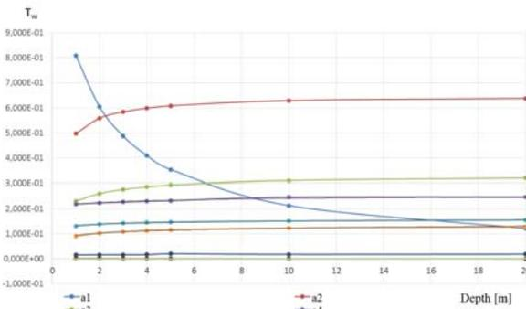
Fig. 16 Dependencies of relative changes in temperature  $T_w$  on the location depths of the system for the parameters occurring in equation (2).
