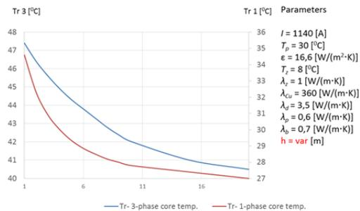
Fig. 17 Temperatures of the three phase cable core and single cable core at various location depths under the ground surface.
