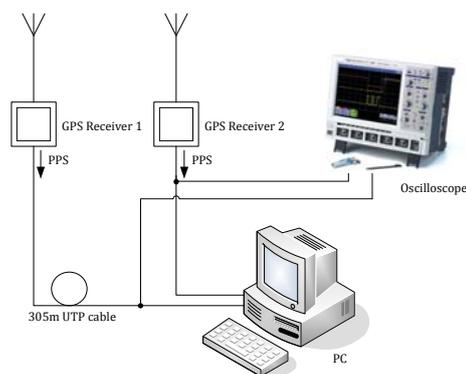
Fig. 5 The configuration III of the measuring system
