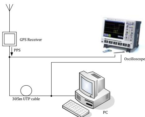
Fig. 3 The configuration II of the measuring system
