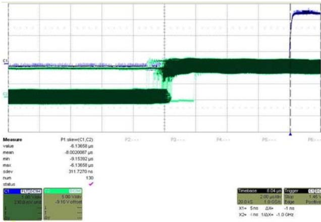
Fig. 8. Results of time-delay of the PPS signal passing through the T208 switch [12]
