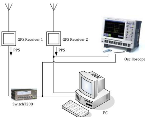
Fig. 7. Configuration of the measuring system with the Westermo T208 switch
