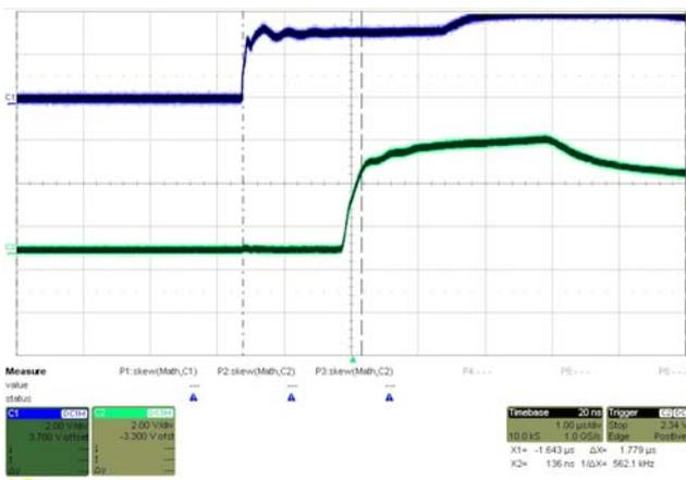
Fig. 4 Results of time-delay of PPS signal in UTP cable of 305 m length obtained in the measuring system from Fig. 3 [12]
