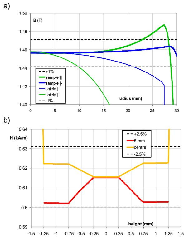
Fig.11. Distribution of  $B$  (a) and  $H$  (b) in the optimised three-lamination ellipsoid at high excitation, 15 kA-t (configuration from Fig. 10)
