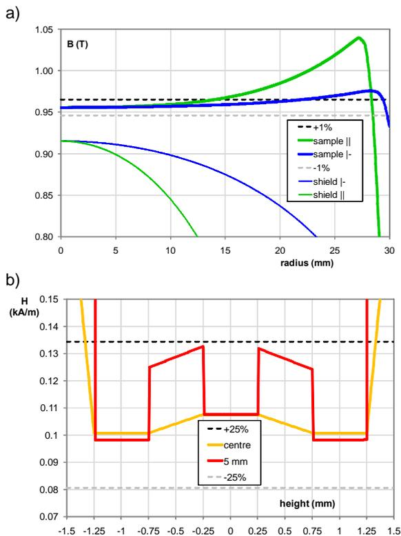
Fig.12. Distribution of  $B$  (a) and  $H$  (b) in the optimised three-lamination ellipsoid at lower excitation, 5 kA-t (configuration from Fig. 10) – compare with Fig. 11
