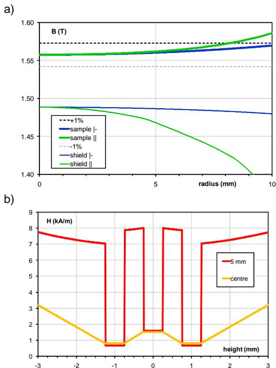
Fig.9. Distribution of  $B$  (a) and  $H$  (b) in the three-lamination ellipsoid at high excitation, 15 kA-t (configuration from Fig. 2c,d,e)
