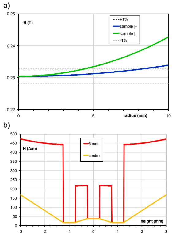
Fig.8. Distribution of  $B$  (a) and  $H$  distribution (b) in the three-lamination ellipsoid at low excitation, 1000 A-t (configuration from Fig. 2c,d,e)
