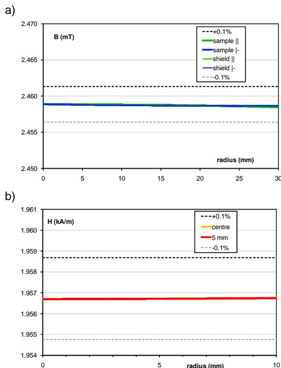
Fig.3. Uniformity of excitation without ferromagnetic laminations: a) distribution of  $B$  – all four lines are on top of each other, b) distribution of  $H$  – both lines are on top of each other
