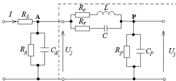
Fig. 1. The equivalent electrical circuit with considering the radiation and convection character
