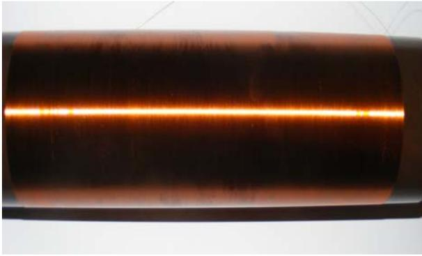
Fig. 4 Wired And painted coil
