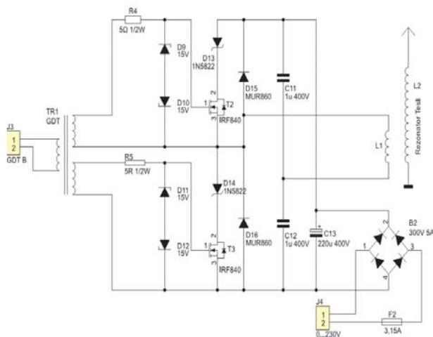
Fig. 1 bridge based on MOSFET's Schema
