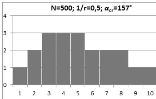
Fig. 5. Histogram of the frequency of arcs of the dislocation line having from 1% to 10% of the length of the total length of the dislocation line, number of defects  $N = 500$ , acting force  $F \sim 0.5$ , critical angle  $\alpha_{cr} = 157^\circ$ .
