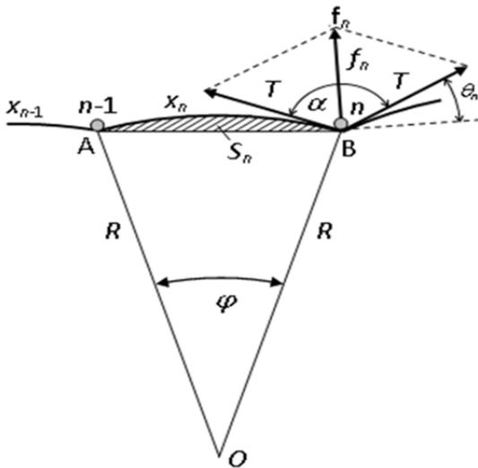
Fig.2. Force  $f_n$  acting by dislocation on the point defect  $n$ ,  $\alpha_n$  - opening angle,  $S_n$  - area occupied by the dislocation before stop.
