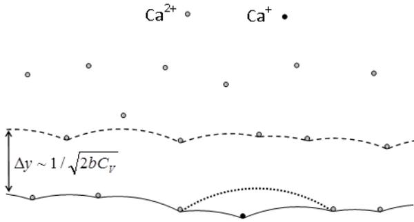
Fig.1. Starting position of the dislocation (solid line) and its position on the second line of obstacles (broken line). Dotted segment represents the first unlocking of the dislocation from the magnetoactive center (black circle) after the magnetic field was switched on and the beginning of the cascade unzipping propagation (to the left and to the right).
