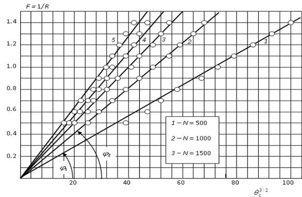
Fig. 3. Dependence of the threshold force  $F_{cr}$  on the critical angle for various numbers of the point defects.
