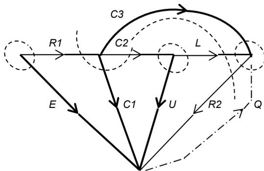
Fig.2. The structural graph  $\Gamma$  of the circuit with the selected branches of the normal tree  $T$  (bolt lines), chords  $N$  (thin lines), principal cutsets (dotted lines), and dot-and-dash chord  $Q$
