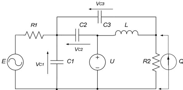
Fig.1. A simple circuit containing a degenerate loop C1-C2-U
